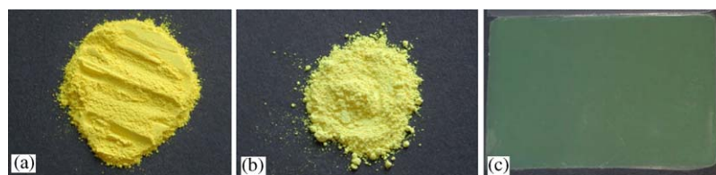
Fig. 1. Color of K_3PMo_{12}O_{40} samples prepared by: (a) the oxide route and (b) the acid route. The hue of a mixture K_3PMo_{12}O_{40} , polypropylene and polyethylene glycol heated at 180 °C is shown in (c).
